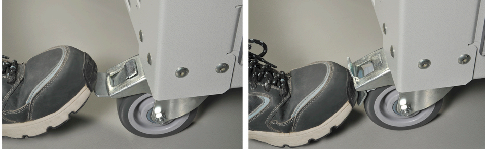
Figure 10. Locking the swivel casters of the Electrical Pitch Hub.
