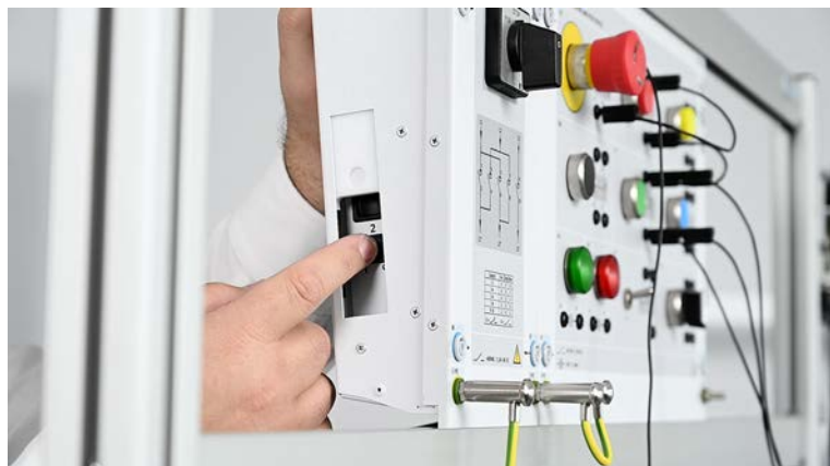
Figure 47: Fault insertion on a module using switches.
