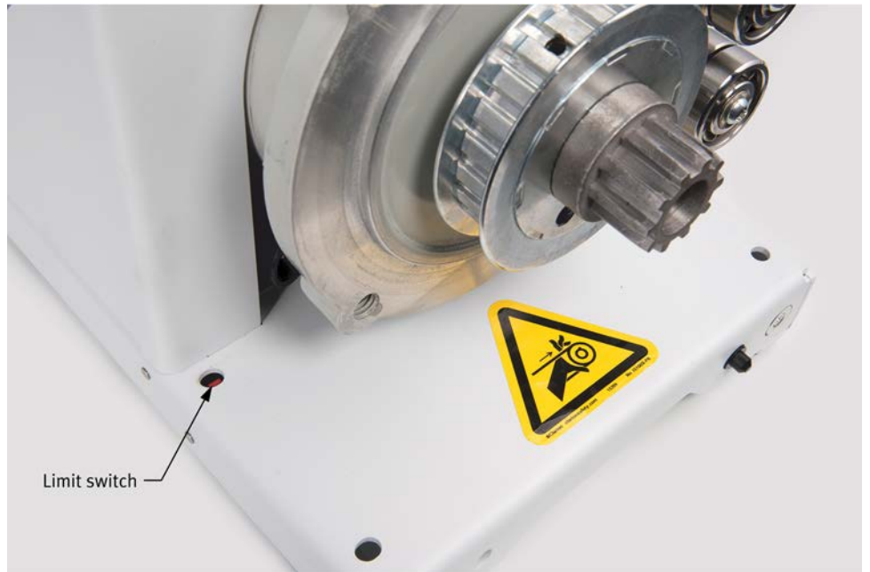
Figure 15: A limit switch in the base plate of each rotating machine prevents machine operation as long as a protective guard is not properly installed.
