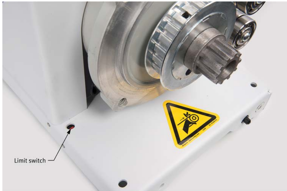
Figure 7: A limit switch in the base plate of each rotating machine prevents machine operation as long as a protective guard is not properly installed.
