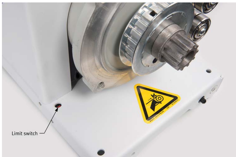
Figure 12: A limit switch in the base plate of each rotating machine prevents machine operation as long as a protective guard is not properly installed.
