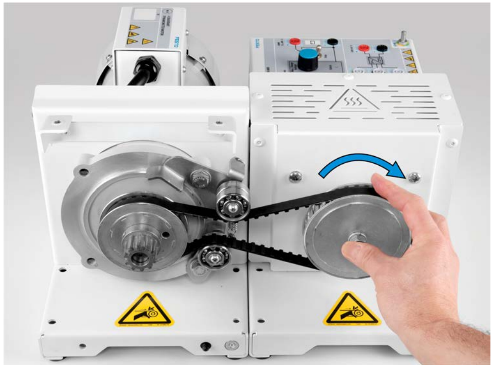
Figure 6: To ensure the timing belt is installed correctly, rotate the shaft of either the prime mover or the rotating machine by hand. Both machines should rotate and tension should be applied to the timing belt by both bearings of the tensioner.
