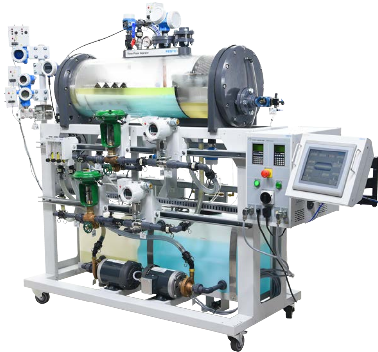
Figure 11: Three-Phase Separator Learning System with Instrumentation.
