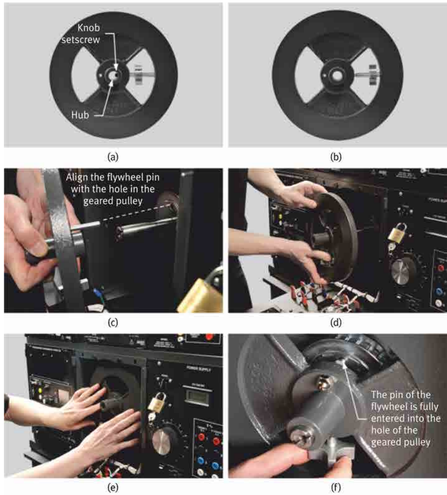
Figure 27: Installing a flywheel on the shaft of an EMS rotating machine.
