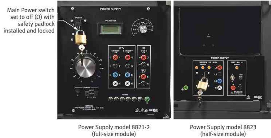
Figure 32: On the Power Supply, make sure that the main power switch is set to the O (off) position. Also, make sure that the safety padlock of the main power switch is installed and locked.
