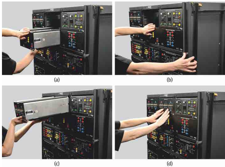
Figure 23: Installing a stack of two half-size EMS modules in a full-height compartment of a workstation.
