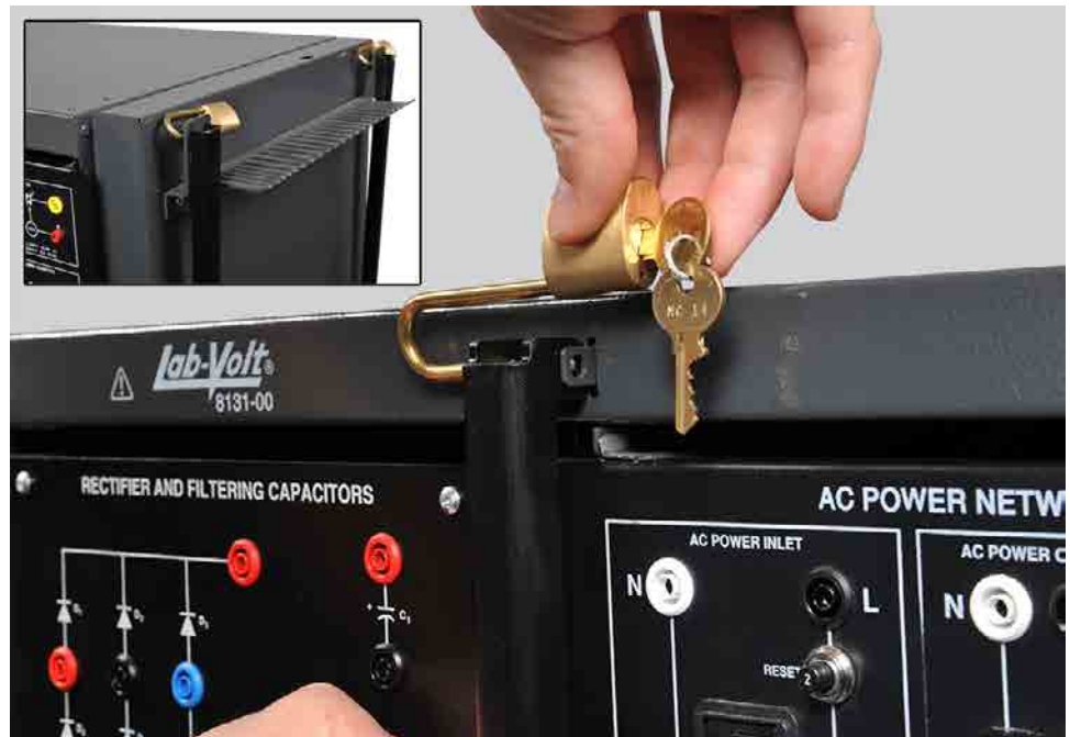
Figure 20: Two safety bars must be padlocked to the front of the workstation to prevent students from removing EMS modules during laboratory exercises. The bars can be removed and padlocked to the side of the workstation when the safety lock is not necessary.
