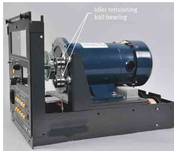
Figure 41: The idler tensioning ball bearings of EMS rotating machines require periodical lubrication.
