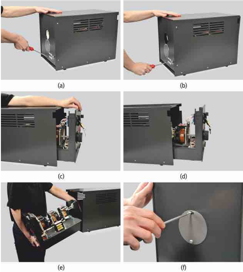
Figure 40: Removing a Power Supply from the Workstation, Model 8133.
