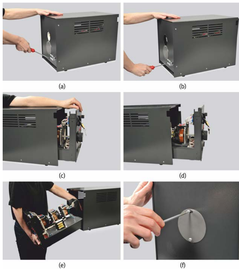
Figure 39: Removing a Power Supply from the Workstation, Model 8133.
