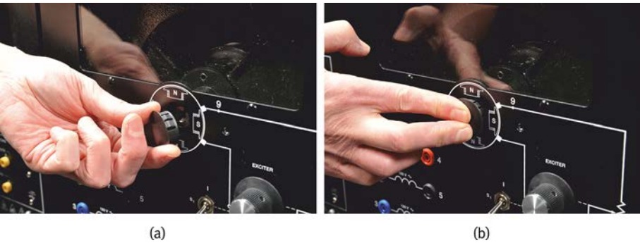
Figure 27: Installing the plastic cap covering the end of the machine shaft.
