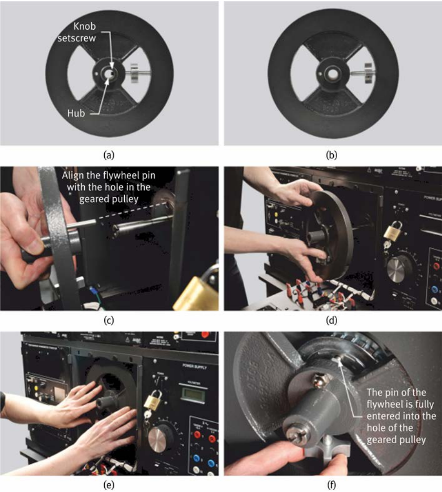
Figure 26: Installing a flywheel on the shaft of an EMS rotating machine.
