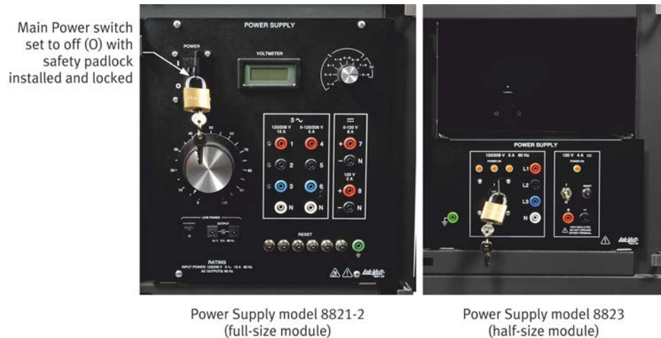
Figure 31: On the Power Supply, make sure that the main power switch is set to the O (off) position. Also, make sure that the safety padlock of the main power switch is installed and locked.
