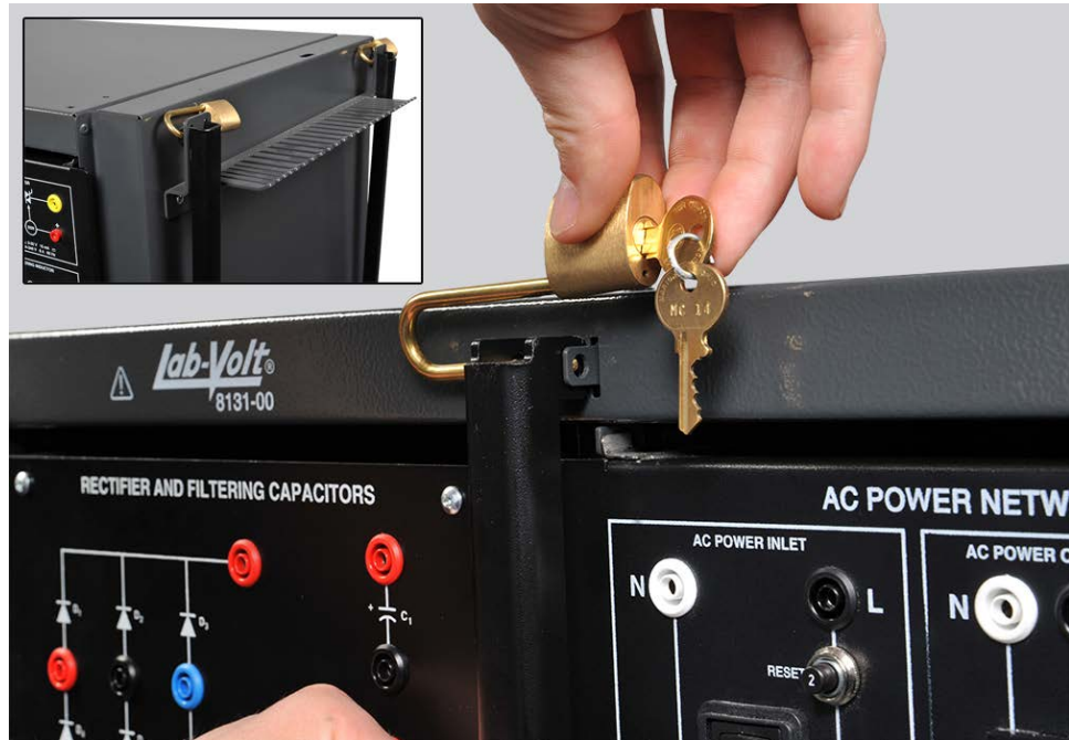
Figure 19: Padlock the two safety bars to the workstation front to prevent students from removing EMS modules during laboratory exercises. When the safety lock is not required, remove the bars and padlock them to the side of the workstation.
