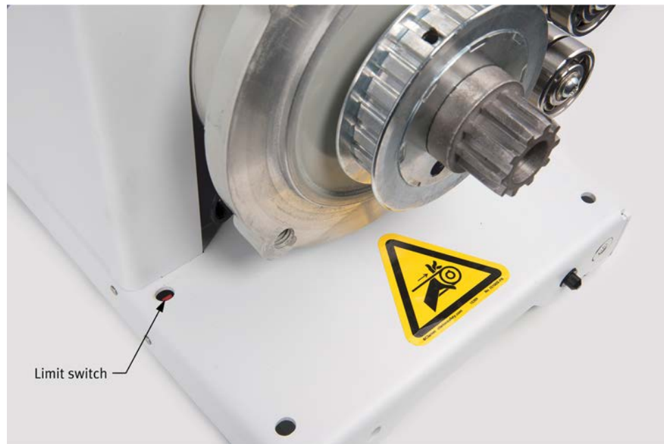
Figure 15: A limit switch in the base plate of each rotating machine prevents operation unless a protective guard is properly installed.
