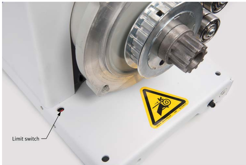
Figure 10: A limit switch in the base plate of each rotating machine prevents machine operation as long as a protective guard is not properly installed.
