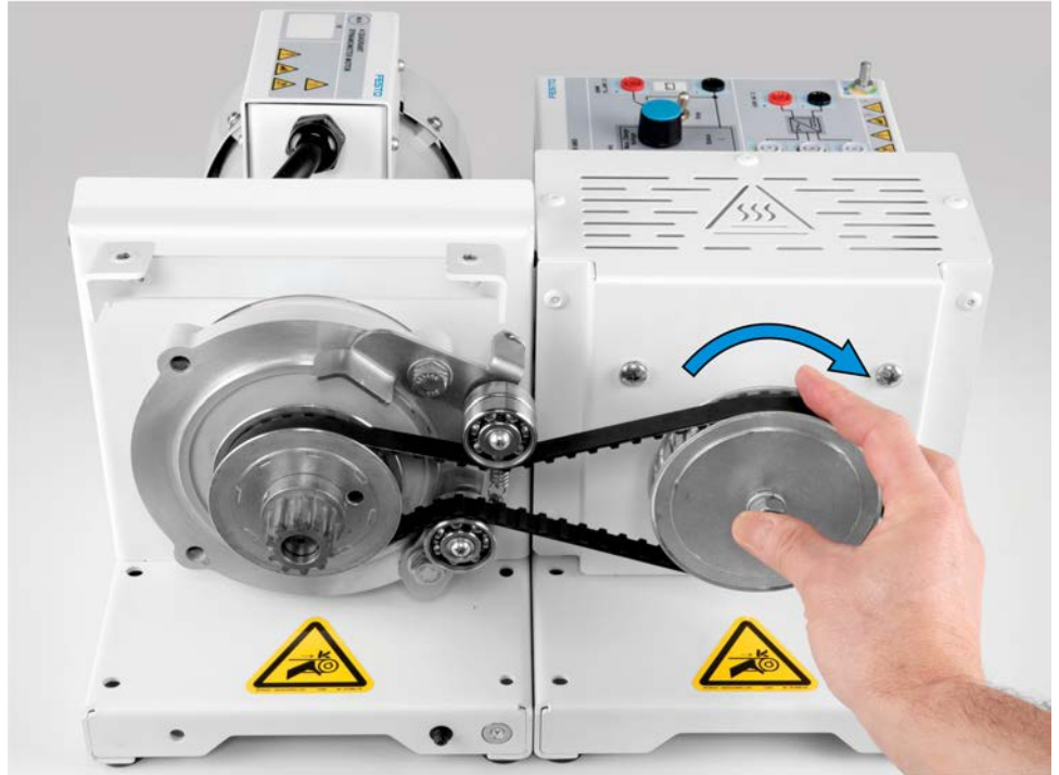
Figure 9: To verify correct installation of the timing belt, rotate the shaft of either the prime mover or the rotating machine by hand. Both machines must rotate, and both tensioner bearings must apply tension to the belt.
