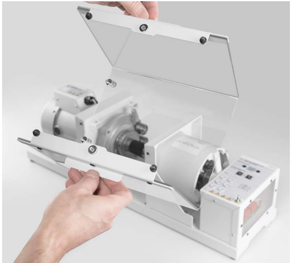
Figure 16: Guiding pins at the bottom of the protective guard for in-line rotating machines.
