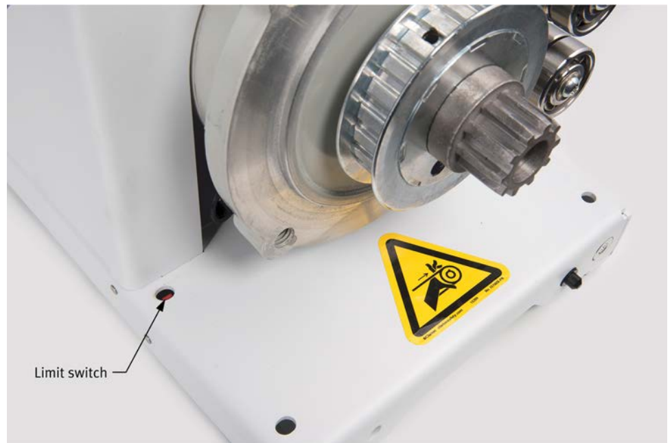
Figure 18: A limit switch in the base plate of each rotating machine prevents operation unless a protective guard is properly installed.
