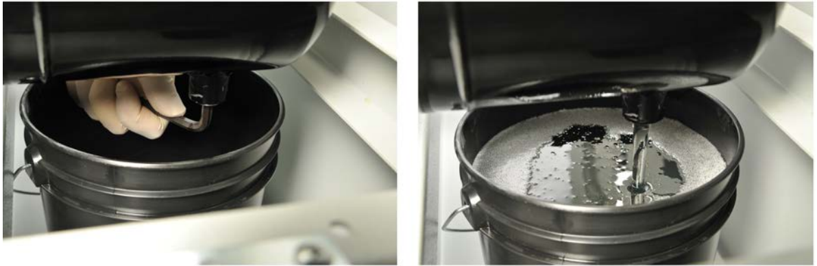
Figure 64: Unscrewing the drain plug.
