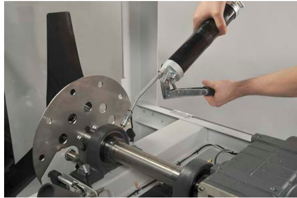
Figure 58: Inserting the grease gun into the pillow block nipple.
