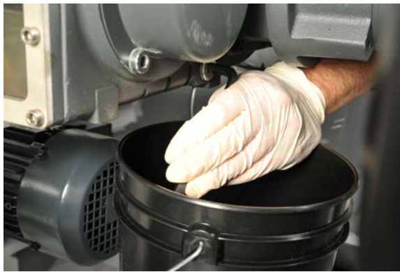
Figure 60: Removing the drain plug.
