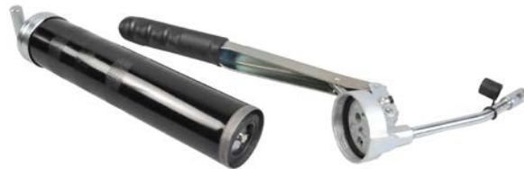
Figure 53: Opening the grease gun.
