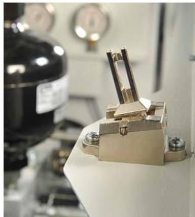
Figure 30: Side doors safety mechanism.
