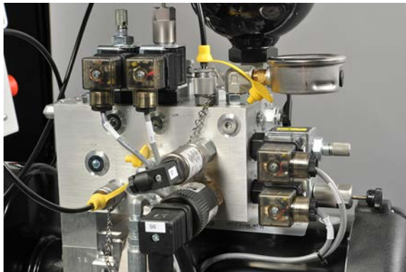
Figure 27: The solenoids of the hydraulic unit can get hot.
