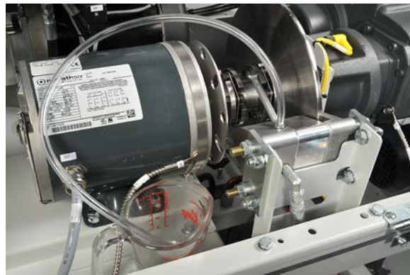
Figure 68: Preparing to bleed the rotor brake.
