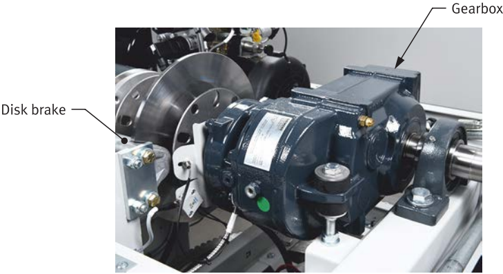
Figure 6: Gearbox and disk brake.
