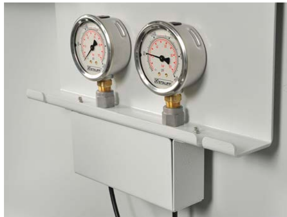
Figure 9: Hydraulic pressure gauges.
