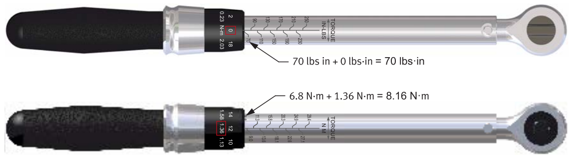
Figure 50: Examples of wrench adjustments (Metric and SAE).
