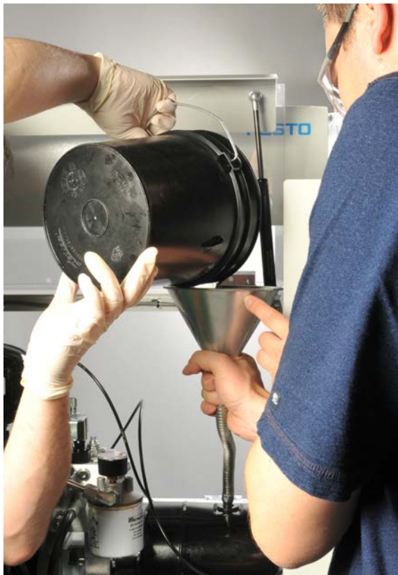
Figure 67: Filling up the hydraulic oil tank.
