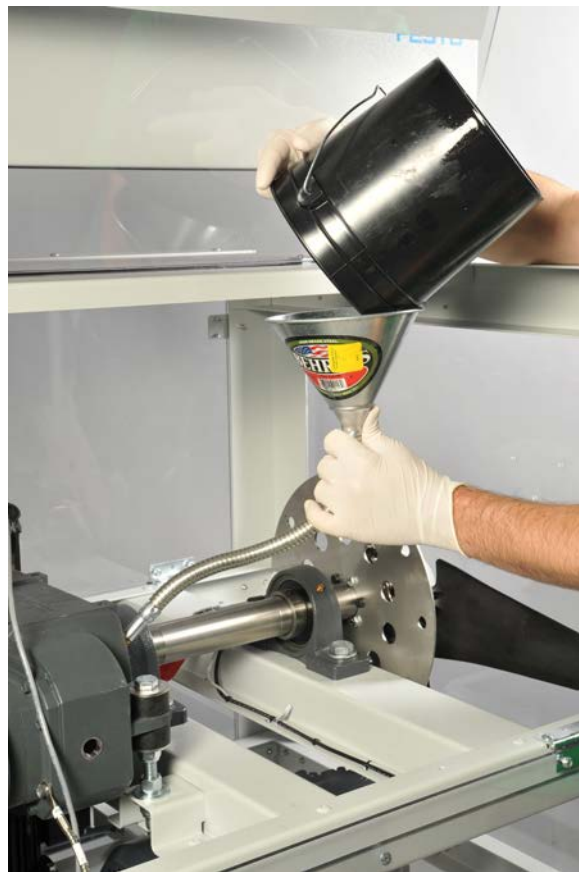
Figure 62: Pouring new oil into the gearbox.
