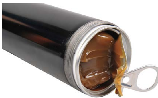
Figure 56: Removing the seal.
