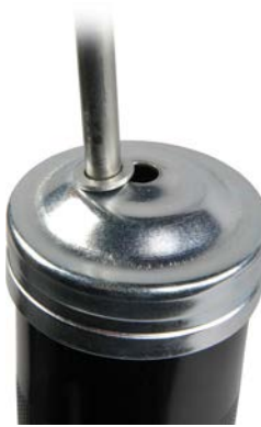
Figure 52: Locking the rod handle.
