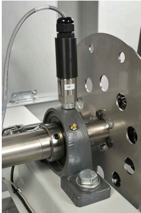
Figure 45: Never let the vibration sensor cable run near moving parts as it could be stuck and become damaged.
