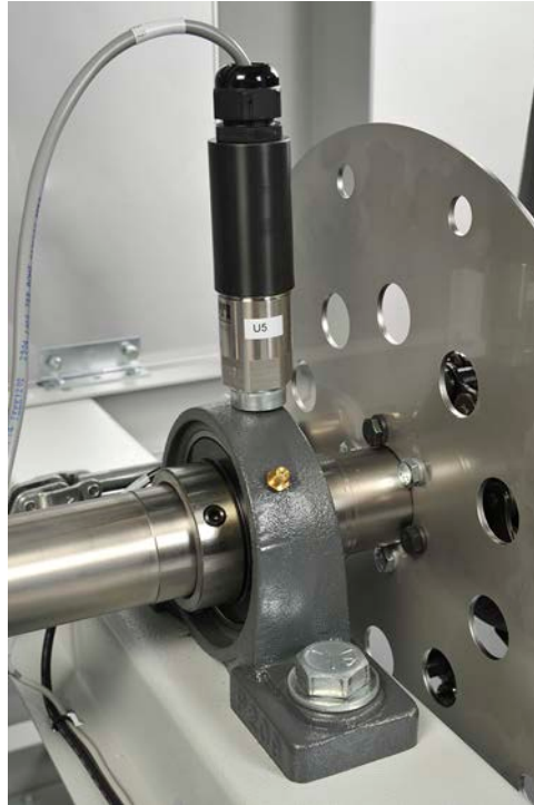
Figure 41: Never let the vibration sensor cable run near moving parts as it could be stuck and become damaged.
