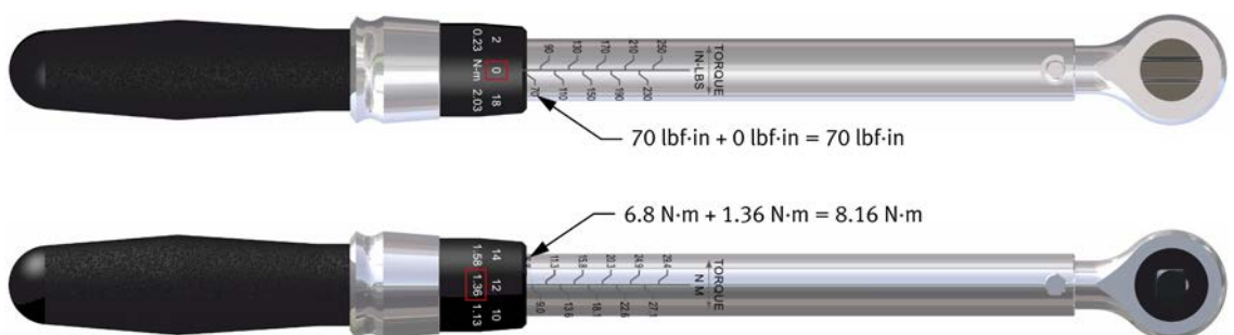
Figure 46: Examples of wrench adjustments (Metric and SAE).
