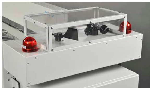
Figure 29: Measuring equipment enclosure.
