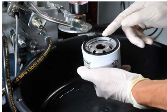
Figure 62: Coating the filter seal with oil.
