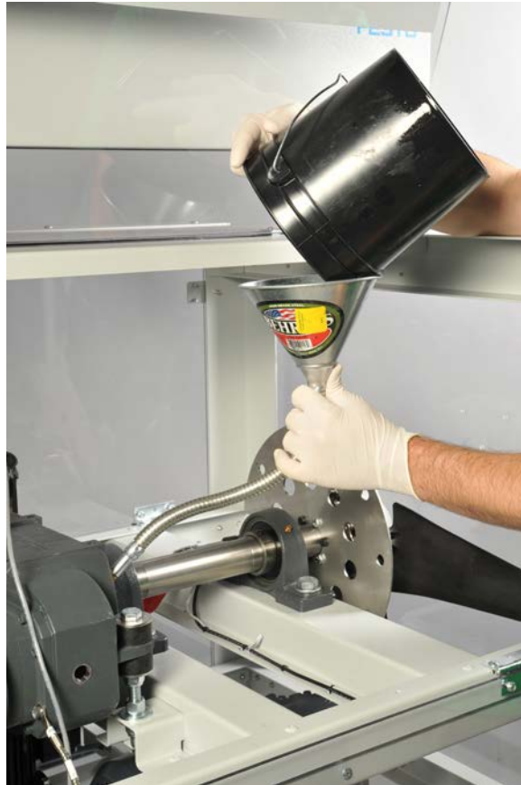
Figure 58: Pouring new oil into the gearbox.
