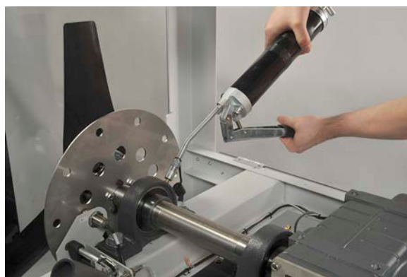
Figure 54: Inserting the grease gun into the pillow block nipple.
