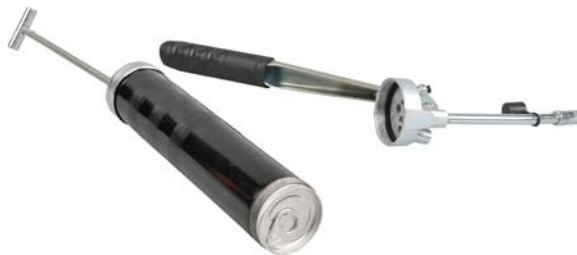
Figure 51: Inserting a new grease cartridge.
