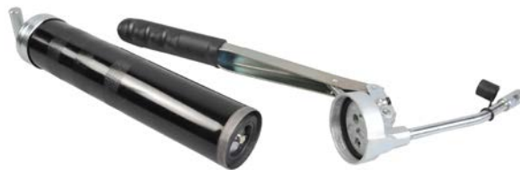
Figure 49: Opening the grease gun.
