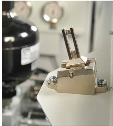
Figure 26: Side doors safety mechanism.
