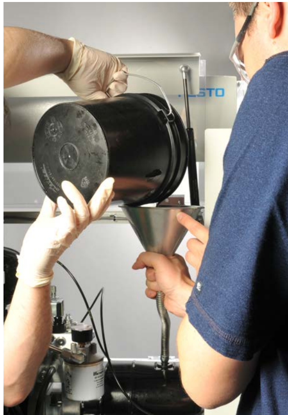
Figure 63: Filling up the hydraulic oil tank.
