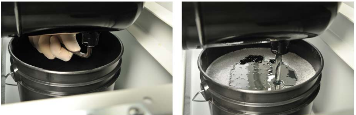
Figure 60: Unscrewing the drain plug.
