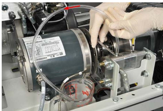
Figure 65: Oil flowing out of the rotor brake caliper.
