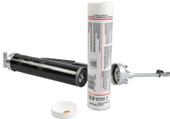
Figure 50: Removing the plastic cap.
