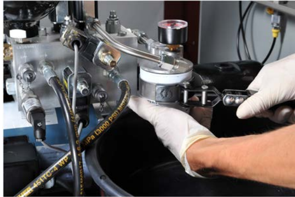
Figure 61: Removing the oil filter.
