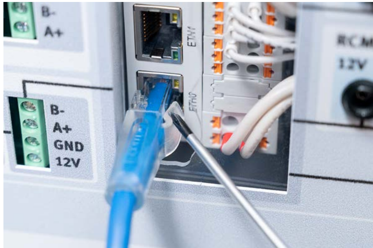
Figure 3: To remove the Ethernet cable, you may need to use a small screwdriver to push on the tab.
