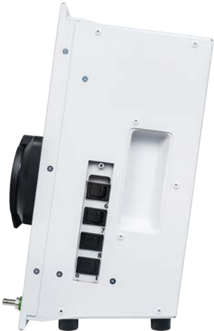
Figure 12: Fault switches on the side of a module.
