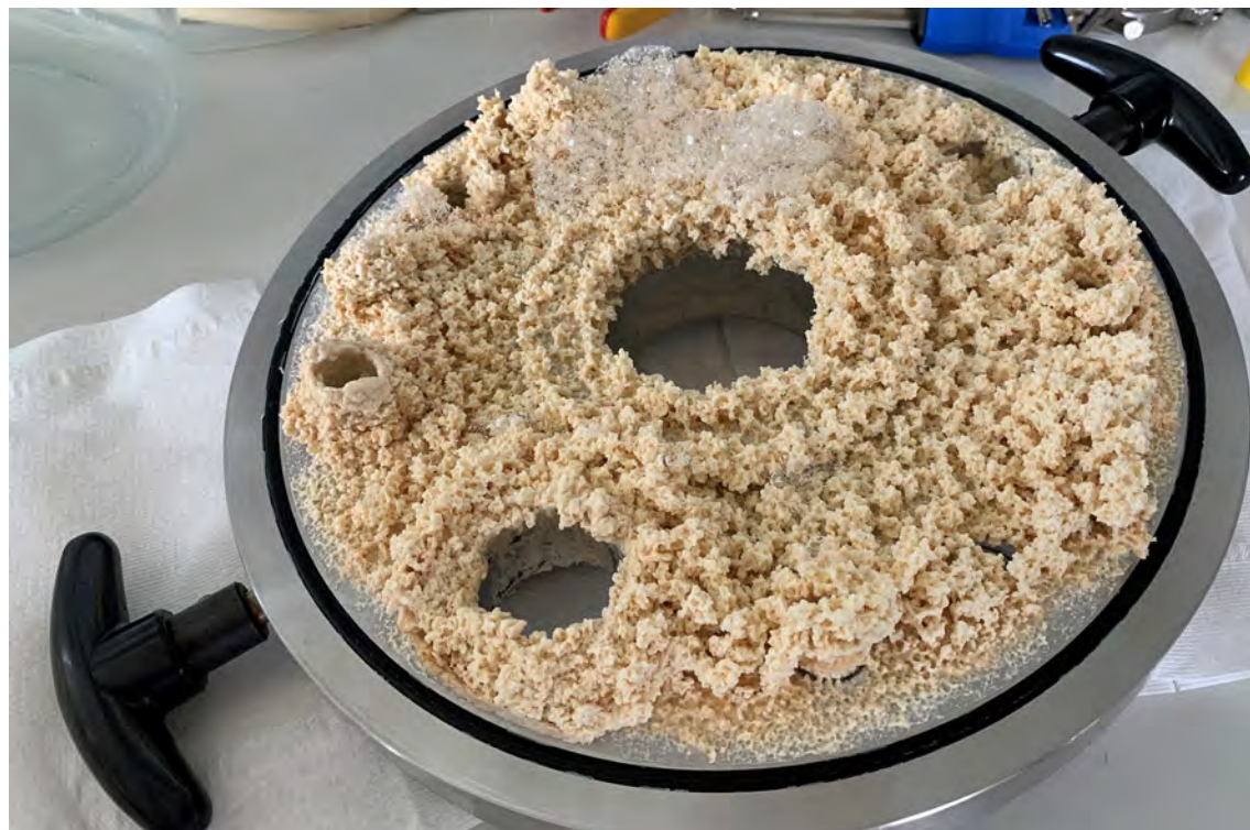
Bioreactor headplate after CL fermentation with persistent foam deposits Source: Amira Oraby
