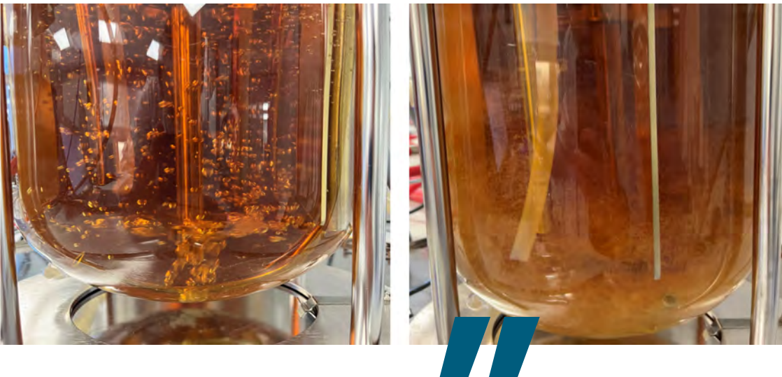
Coarse bubbles produced by conventional stainless-steel tubes (left) versus fine bubbles produced by porous materials (right) for the aeration of culture broth.
