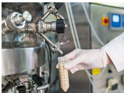
Left: Sampling of MEL fermentation broth from a 75-L-bioreactor. Right: Purified mannosylerythritol lipid for application testing
