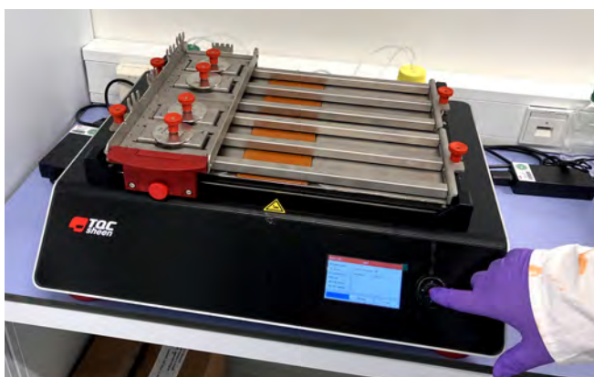
TQC Sheen multi-track wiper employed for standardized cleaning performance testing of all-purpose cleaners.
