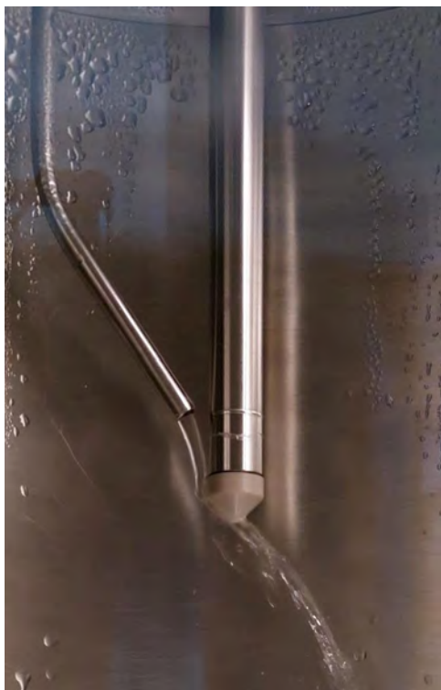
LMT105 sensor during test run (sensitive zone in beige polymer), flushed with clear water to simulate inline cleaning Source: Amira Oraby
