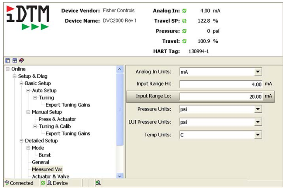
Figure 22: Configuring the DVC2000 to reverse the action of the valve.
