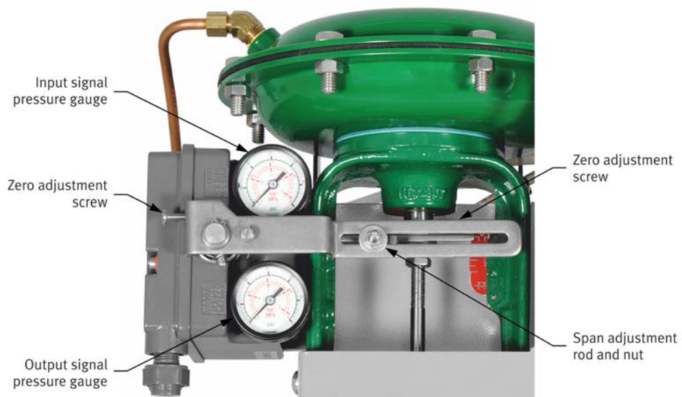
Figure 15: Front view of a valve with a positioner.
