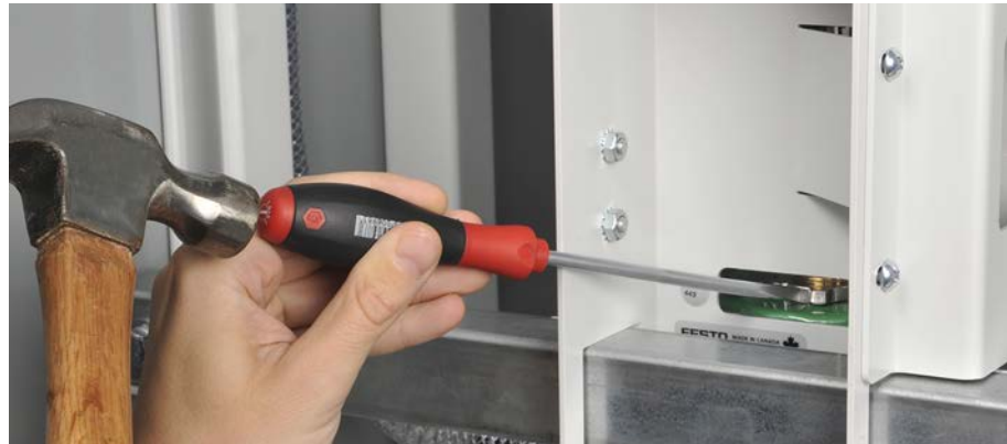
Figure 10: Unscrewing the actuator locknut to loosen the valve body.
