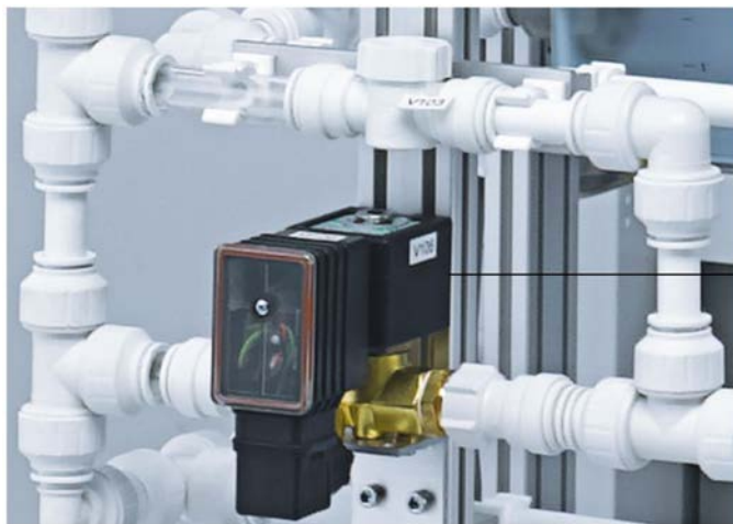
Figure 9: Controlling element proportional valve V106.
