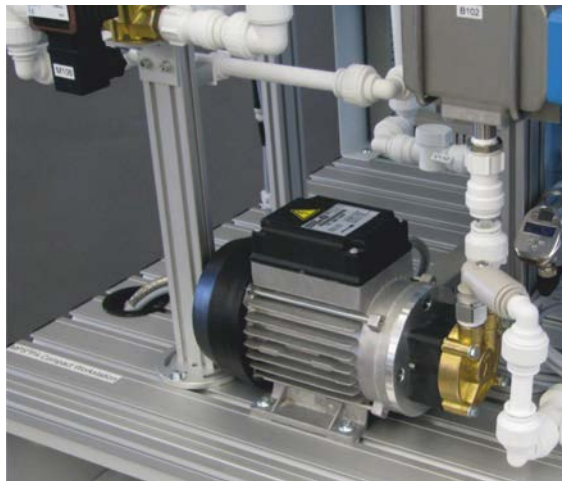
Figure 33: Centrifugal pump with 3-phase AC-motor - for illustration only.
