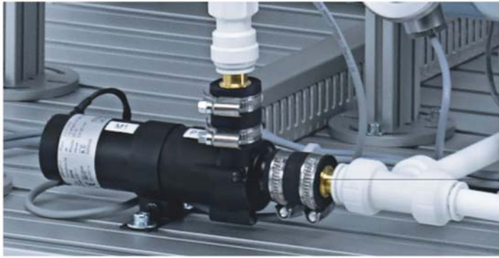
Figure 8: Controlling equipment – Pump P101 (1).
