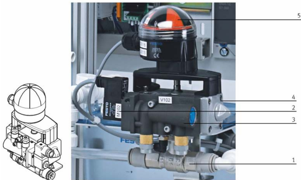
Figure 13: 2-way ball valve V102 with pneumatical rotary drive.
