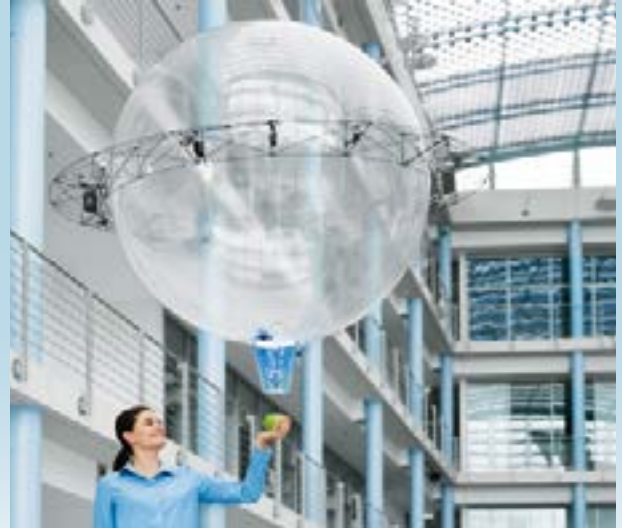
FreeMotionHandling: Autonom fliegende Greiferkugel FreeMotionHandling: Autonomously flying gripping sphere
