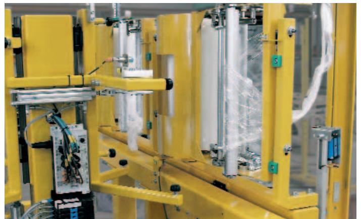
Quick change: Controlled by a CPX/MPA, Festo drives provide fully-automatic replacement of an empty sheeting magazine by a full one.
