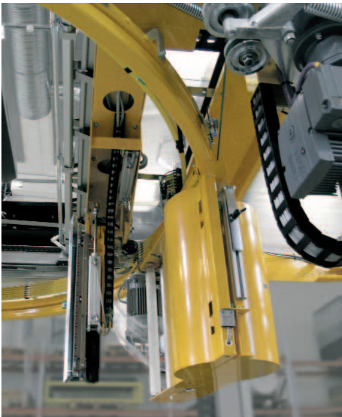
Quick change: Controlled by a CPX/MPA, Festo drives provide fully-automatic replacement of an empty sheeting magazine by a full one.
