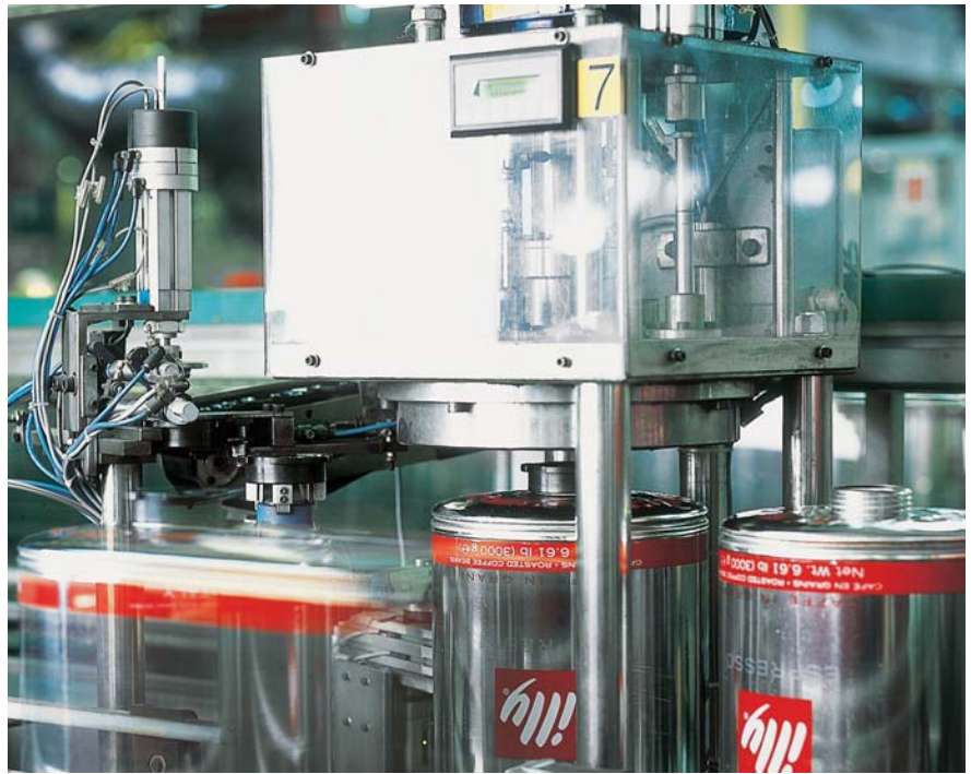
Perfect handling: Air is extracted from the cans and replaced by inert gas. The cans are then sealed with plastic lids.
