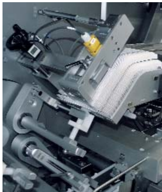
Before: complicated carton separating with cam disk.
