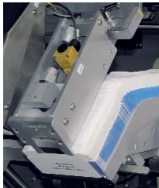
After: fast carton separation with MAS pneumatic muscle.
