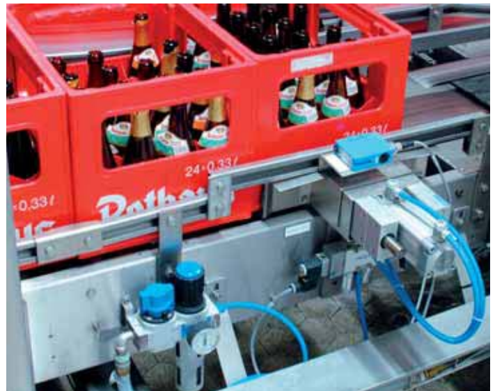
From process to factory automation: Pneumatic valve terminals and drives are in their element not only in the brewing process, but also in bottling and packaging.
