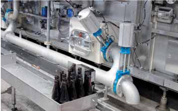
DLP valve actuators from Festo: In the Innoclean bottle washing machine by KHS for opening and closing gate valves supplying cleaning fluid
