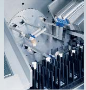
3 The blister packs are stacked in slots in the lane for goods to be packaged in the cartoner. At the same time, collapsible cardboard boxes are pulled, set up and placed onto a second lane behind the blister packs.
