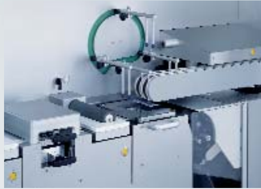
2 Faulty blister packs – recognised by the camera – are identified with a special stamped contour at the stamping station and are removed from the packaging process.
