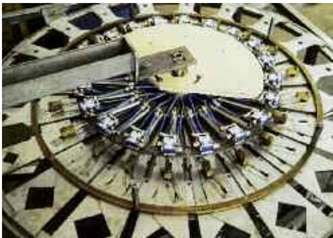
Top: Finger-tip touch – inserting the artichoke buds into the clamping disc.
