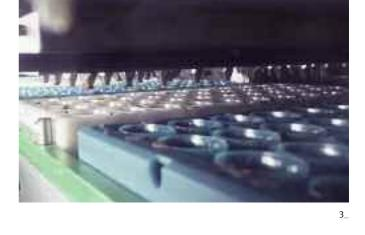
the next step, the chocolate mass is evenly distributed in the cavities by stamps pressed in from above which have been cooled down to 23 degrees. In order to maintain a constant air humidty of 2 % and to prevent sticking of the ice-cold stamps and hot chocolate due to condensed water, an air supply pipe continually blows dried air into the station. The next step is to "debur" the moulded edges: Two heated rollers remove the surplus chocolate from the moulds and convey this to a container.
