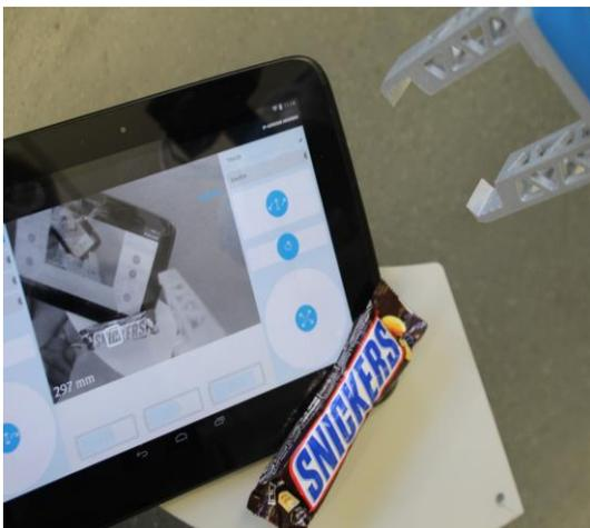
The app to control the robot also displays the distance to the selected object (Snickers).
