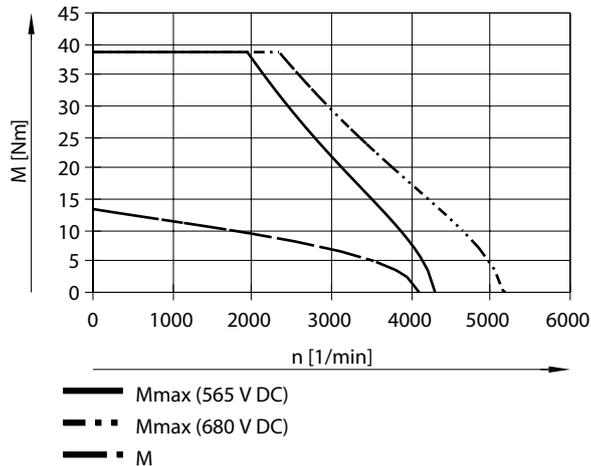
Typical motor characteristic curve at nominal voltage and optimal motor controller. Note the max. permissible rotational speeds of add-on and installation components (such as brake, encoder, etc.).
