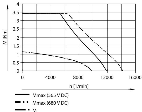
Typical motor characteristic curve at nominal voltage and optimal motor controller.
