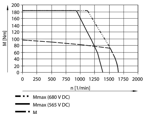
Typical motor characteristic curve at nominal voltage and optimal motor controller. Note the max. permissible rotational speeds of mounting and installation components (such as brake, encoder, etc.).
