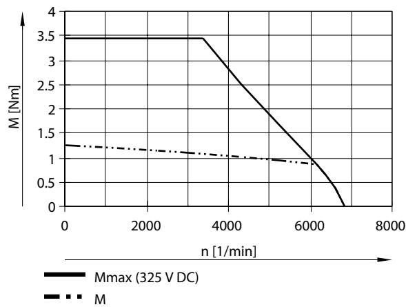
Typical motor characteristic curve at nominal voltage and optimal motor controller.
