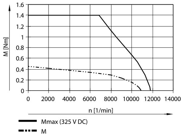
Typical motor characteristic curve with nominal voltage and optimal motor controller.
