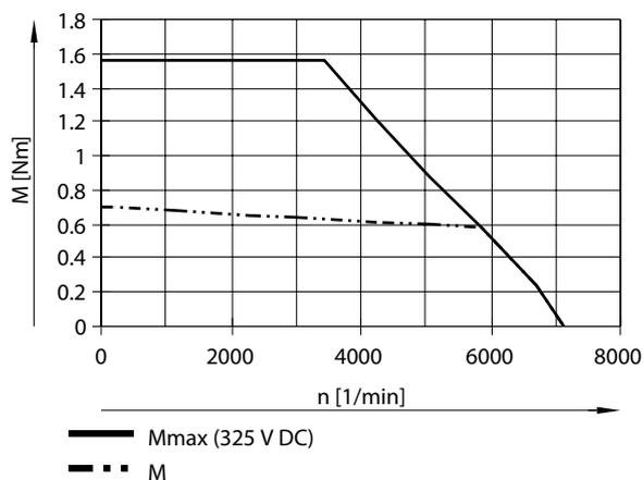
Typical motor characteristic curve at nominal voltage and optimal motor controller. Note the max. permissible rotational speeds of mounting and installation components (such as brake, encoder, etc.).
