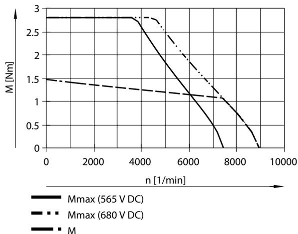
Typical motor characteristic curve at nominal voltage and optimal motor controller. Note the max. permissible rotational speeds of mounting and installation components (such as brake, encoder, etc.).
