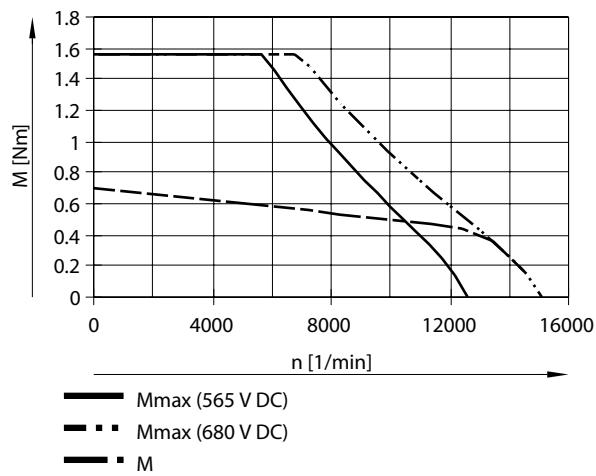
Typical motor characteristic curve at nominal voltage and optimal motor controller.
