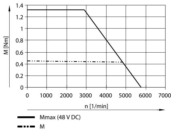
Typical motor characteristic curve with nominal voltage and optimal motor controller.
