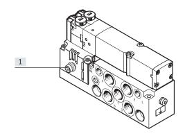
[1] Electrical connection, plug 4-pin, M8, to EN 60947-5-2 Tightening torque for M8 plug: 0.25 ... 0.5 Nm (manual torque)
