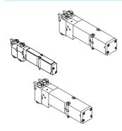
VMPA offers a comprehensive range of valve functions. All valves have a patented sealing system, which ensures efficient sealing, a broad pressure range and a long service life. They have a pneumatic pilot control for optimising performance.
