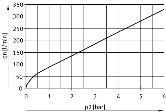
Flow rate q_n as a function of output pressure p_2 , VPPE-3-1-1/8-6-..., q_n 2 -> 3
