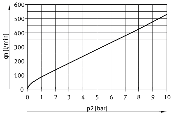
Flow rate q_n as a function of output pressure p_2 , VPPE-3-1-1/8-10-..., q_n 2 \rightarrow 3
