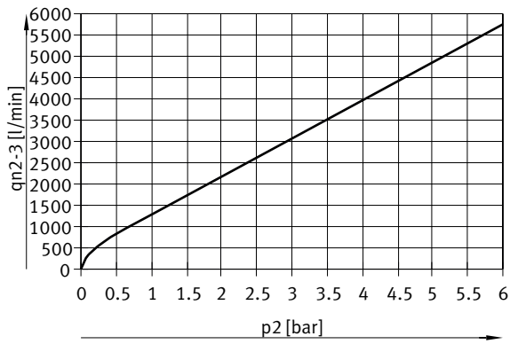
Flow rate q_{n2-3} from 2 -> 3 as a function of excess output pressure p_2 , VPPM-12L-...-0L6H-... (8 bar)
