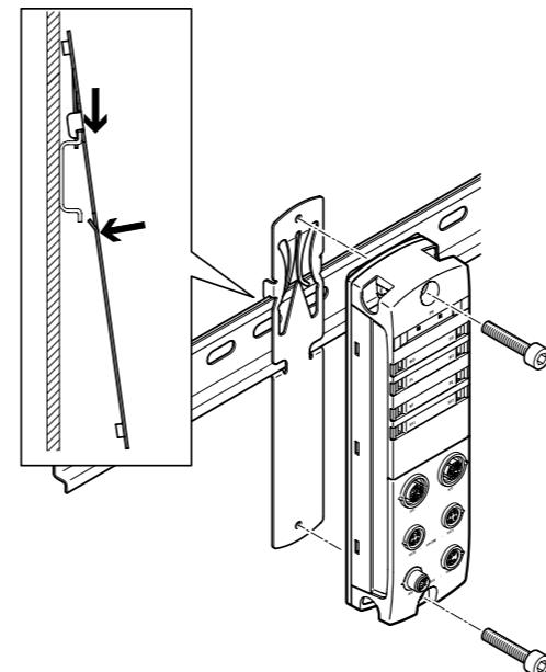
The modules can be mounted on DIN rails according to EN 60715 using the DIN rail mounting CAFM. Two screws with metric thread M4 and correctly sized washers (not included in the scope of delivery) are needed for securing mounting.
