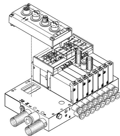
The electrical interfaces are mounted directly on the valve terminal.
