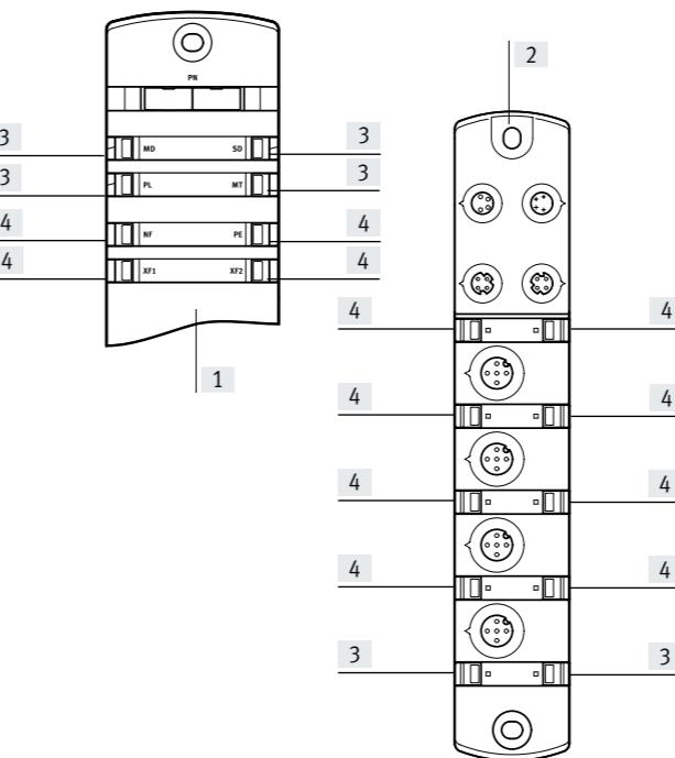
Each module has a row of LEDs for indicating the operating status of the module and of the connected sensors or actuators.
