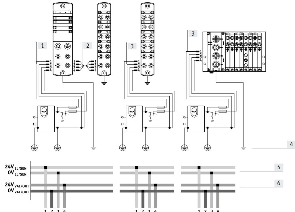
In principle, the remote I/O system CPX-AP-I has two separate electrical circuits:
