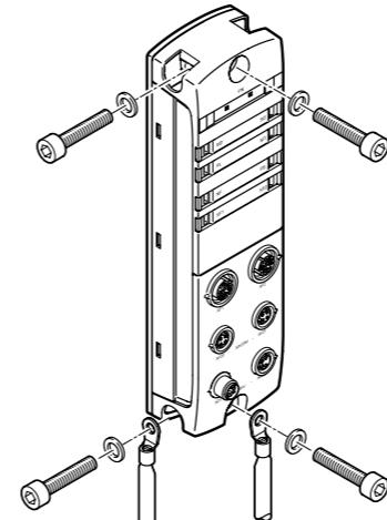
The modules can be mounted on flat surfaces in almost any position using the mounting holes provided (with screws up to 4 mm in diameter). Two screws with correctly sized washers (not included in the scope of delivery) are needed for secure mounting.
