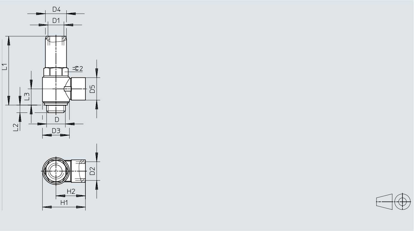
Dimensions – Threaded connection HGL-1/2-B
