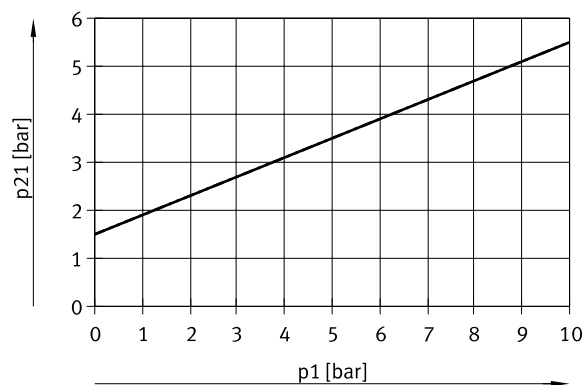
Minimum pilot pressure p_{21} as a function of operating pressure p_1
