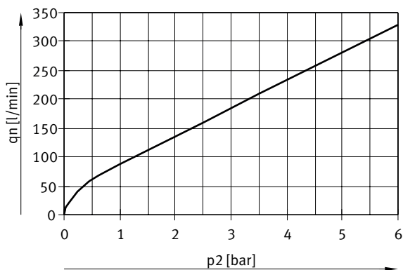
Flow rate q_n as a function of outlet pressure p_2 , VPPE-3-1-1/8-6-..., q_n 2 -> 3
