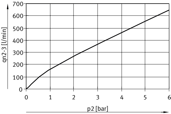
VPPI-5, flow rate q_n for valves with pressure control range 0 ... 6 bar, flow direction 2 > 3; depending on the outlet pressure p_2
