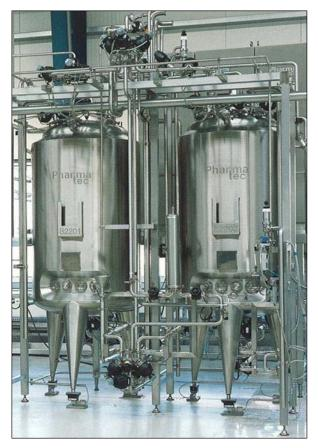
Figure 11: Formulation system in a pharmaceutical application
