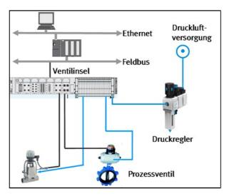
Figure 1: Pneumatic automation architecture
