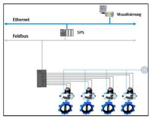
Figure 3: System automation architecture with individual valves
