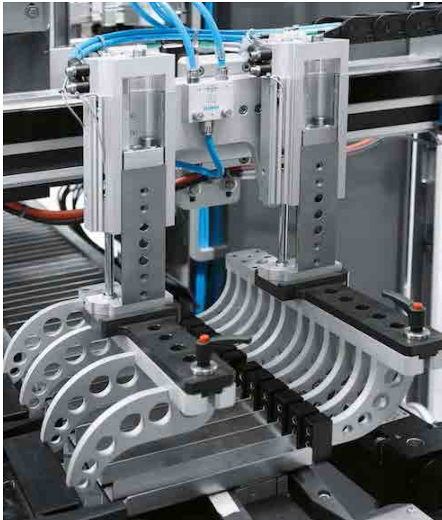
Figure 10: Two Festo DGSL mini-slides mounted on an EGC electric axis in the side loading unit of a state of the art packaging machine
