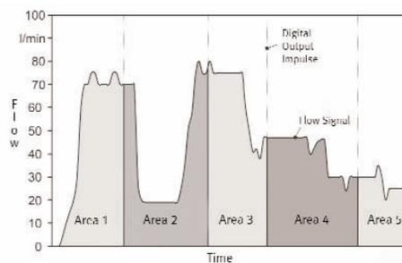
**Figure 4:** Graphical representation of the generation of digital output signals, areas 1 to 5 are all of the same size
