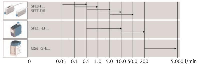
**Figure 3:** The measuring ranges of SFE3/SFET, SFE1 and MS6-SFE
