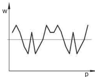
Repetition accuracy is the spread within which the fluidic output quantity is distributed when the same electrical signal, coming from the same direction, is repeatedly selected. Repetition accuracy is expressed as a percentage of the maximum fluidic output signal.
