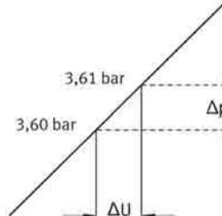
How precisely pressure can be changed, i.e. adjusted, is dictated by the respective device's response sensitivity. The smallest setpoint difference which actually results in a change to output pressure is known as response sensitivity. In this case, response sensitivity is 0.01 bar.
