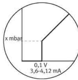
In practice, it may happen that a residual voltage or a residual current is applied to the setpoint input of the VPPM via the setpoint transmitter. Zero suppression is used in order to ensure that, with a setpoint of zero, the valve exhausts the system reliably.
