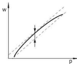
Perfect linearity for the output pressure control characteristic is only possible in theory. Maximum deviation from this theoretical control characteristic, expressed as a percentage, is known as linearity error. The percentage value is relative to maximum output pressure (full scale).
