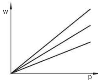
In new condition, 100% setpoint corresponds to 100% of the fluidic output signal. Pressure range adjustment makes it possible to adapt the fluidic output variable to the setpoint.
