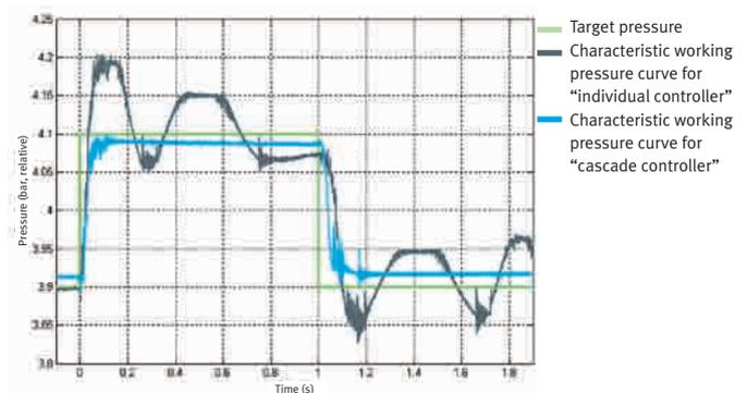
Stable control: close to the ideal characteristic curve with multi-sensor control
