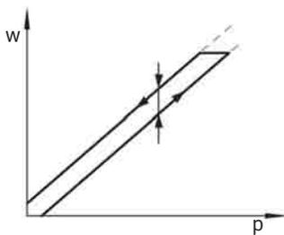
There's always a linear relationship, which lies within a given tolerance, between the specified setpoint and output pressure. It nevertheless makes a difference whether the setpoint is entered in a rising or a falling manner. The difference between the maximum deviation values is called hysteresis.
