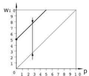
When it is not permissible for a VPPM to exhaust the system, for example due to safety considerations, minimum pressure can be shifted upward from the zero point. An output pressure of, for example, 5 bar is then assigned to the smallest setpoint, and 10 bar to the largest setpoint. If zero offset is used, zero suppression is automatically disabled.
