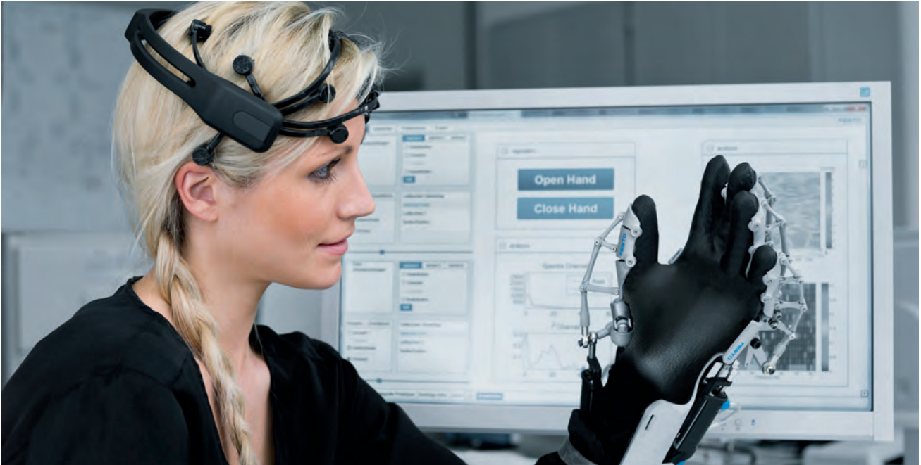
Training for the brain and muscles: the ExoHand in combination with a brain-computer interface
