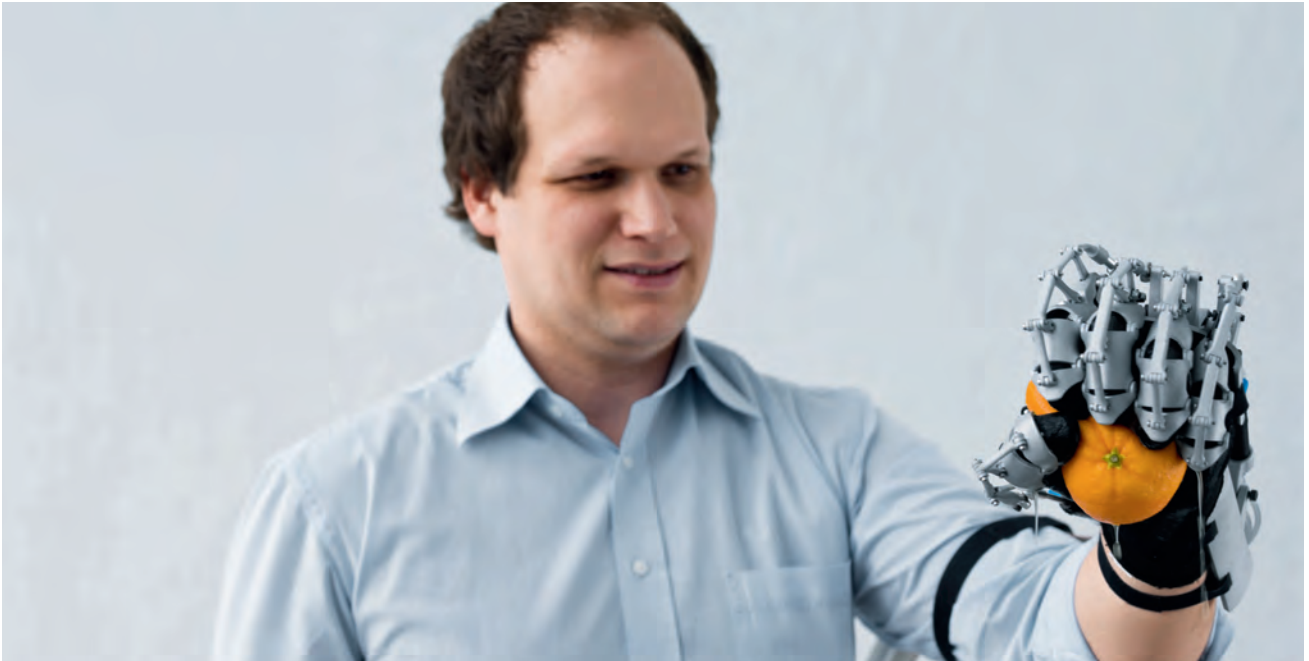
Power assistance: pneumatic actuators for increased gripping force
