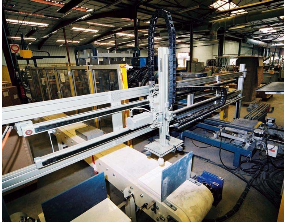
Figure 3: Pick-and-Place systems with toothed-belt actuators are ideal applications for stepper motors and drives
