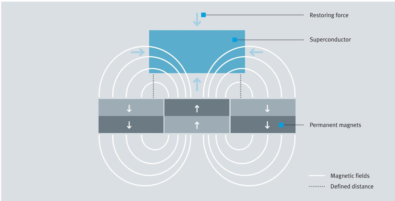
**High-temperature superconductors:** At a transition temperature of  $-196^{\circ}$  Celsius, they store the magnetic field of the permanent magnets at a defined distance.
