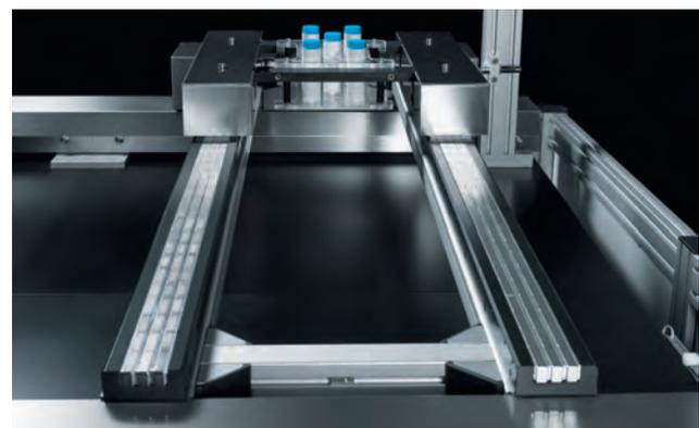
... of an X/Y-table to move on superconductive bearings for the first time.
