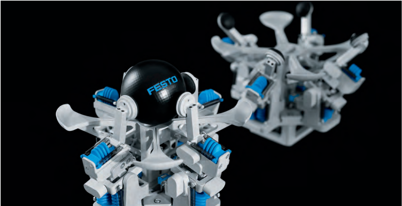
LearningGripper: self-learning gripper system for positioning round objects
