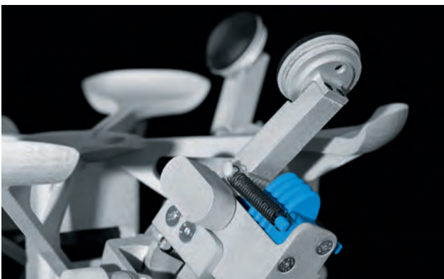
Self-learning: The LearningGripper's four pneumatic fingers ...
