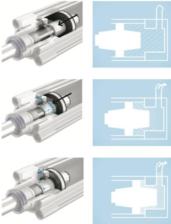
Inside view of a pneumatic cylinder with self-adjusting end-position cushioning PPS moving into the piston end position. Left: the black arrows show the direction of movement of the piston; the blue arrows show the movement of air in the cylinder. Right: air compression and exhaust direction (white hatching and arrows)
