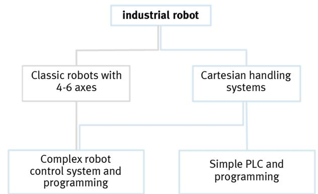
Figure 2: Relationships between robots and control systems
