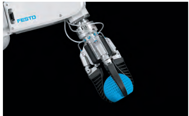
... and the technical application with three adaptive gripping fingers
