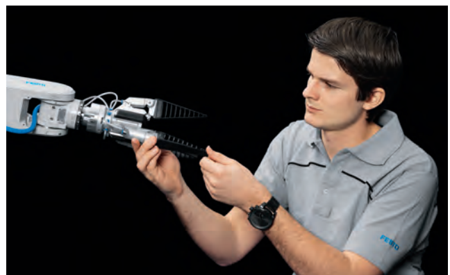
... combined with adaptive fingers with a Fin Ray® structure
