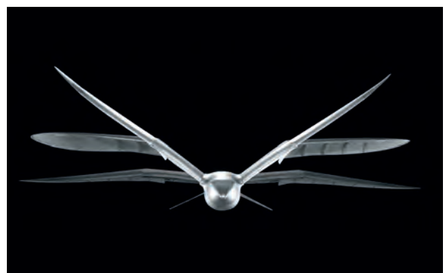
... and active wing rotation modelled on the bionic SmartBird
