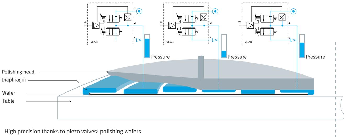
High precision thanks to piezo valves: polishing wafers
