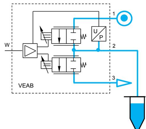
Precise metering, even with very small quantities: piezo valves make adhesive application processes simpler.
