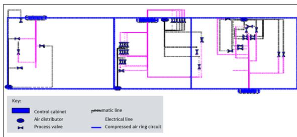
Figure 5: Detailed view of ground level – individual valves
