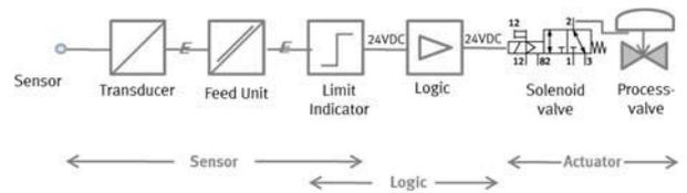
Figure 12: Typical safety instrumented system according to SIL
