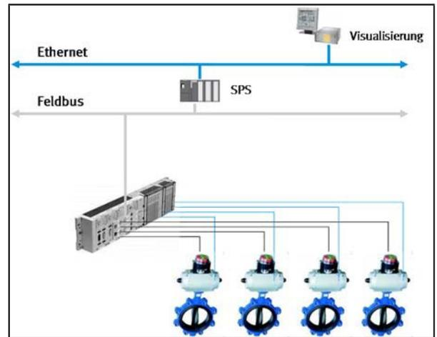
Figure 4: System automation architecture with valve terminal
