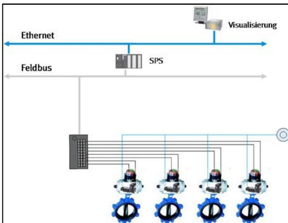
Figure 3: System automation architecture with individual valves
