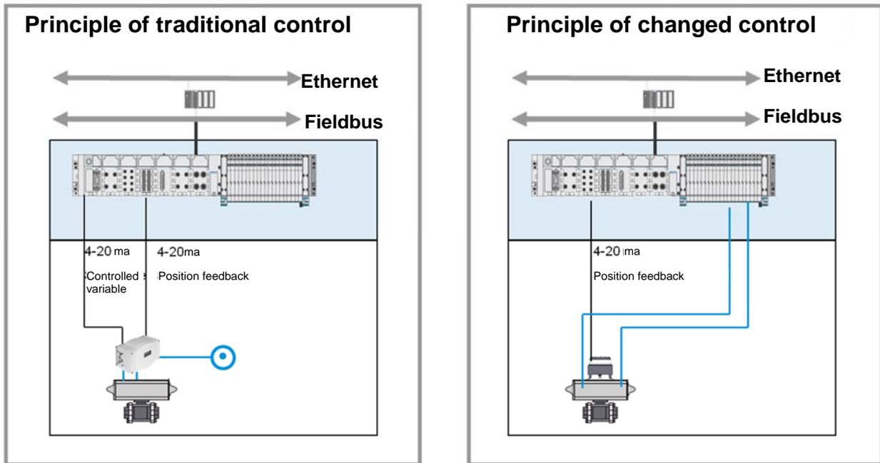
Figure 12: Change in the control circuit structure.
