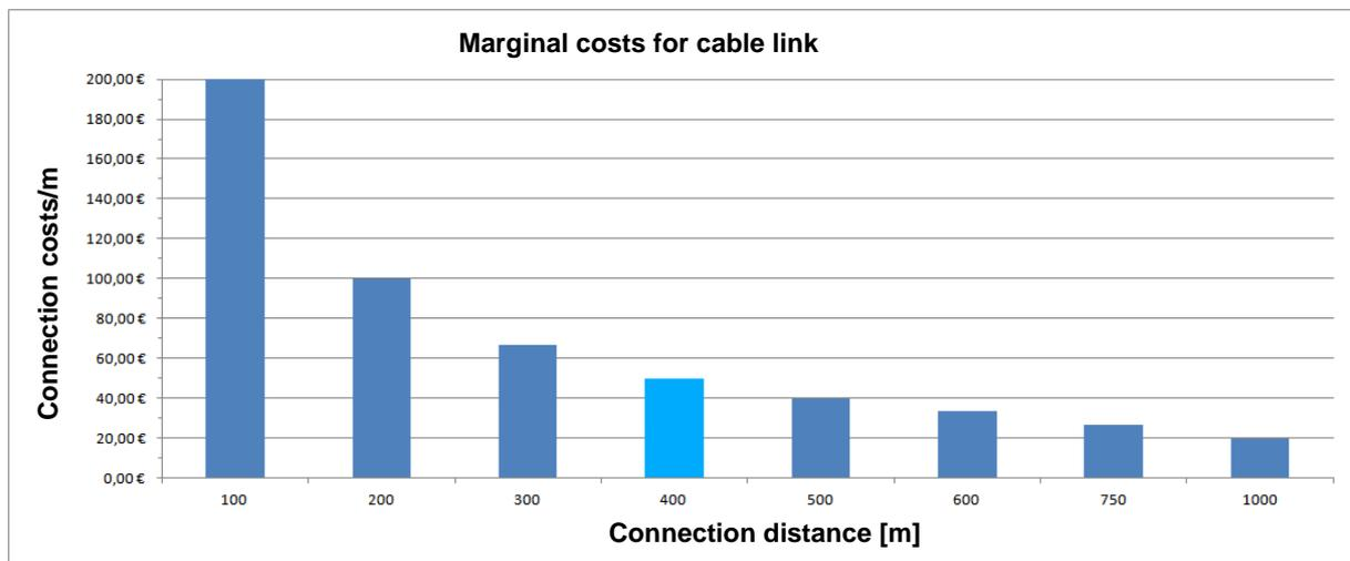
Figure 14: Marginal costs per low-voltage cable to be laid.
