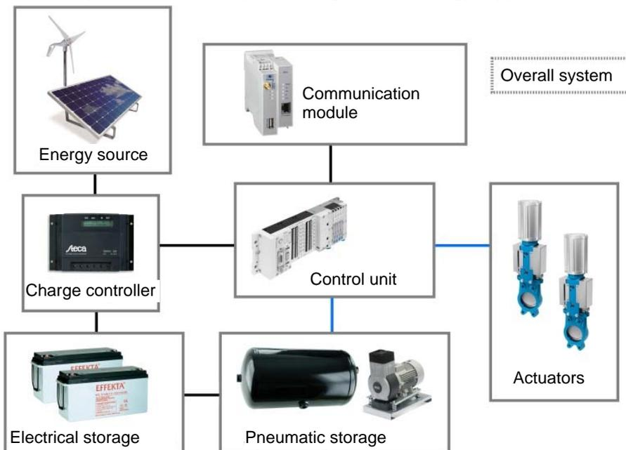
Figure 13: Energy-autonomous automation concept for a rainwater overflow basin in southern Germany.
