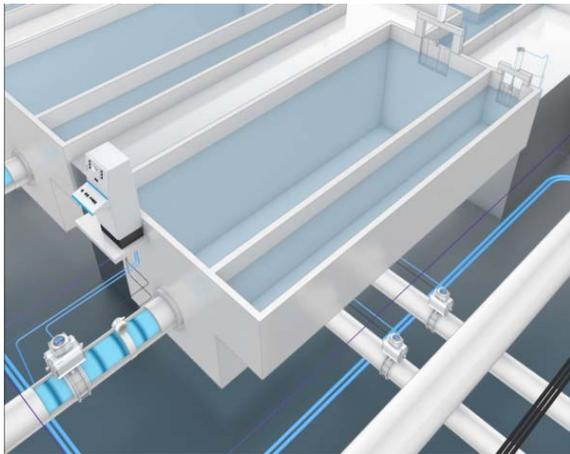
Figure 10: Structure of a solid bed filter.
