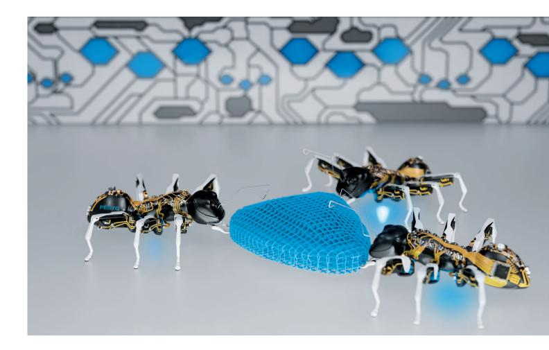
With one eye for detail and the other on the big picture: for the BionicANTs, the Festo engineers have not only taken the delicate anatomy of the natural ant as a role model. For the first time, the cooperative behaviour of the creatures has also been transferred to the world of technology using complex control algorithms.
