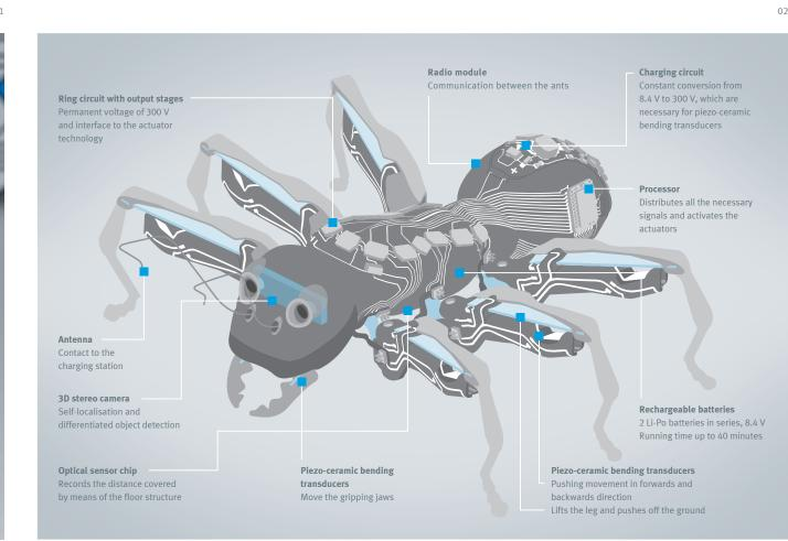
The BionicANTs also come very close to their natural role model in terms of design and constructional layout. Even the mouth instrument used for gripping objects is replicated in very accurate detail. The pincer movement is provided by two piezo-ceramic bending transducers, which are built into the jaw as actuators. If a voltage is applied to the tiny plates, they deflect and pass on the direction of movement mechanically to the gripping jaws.
