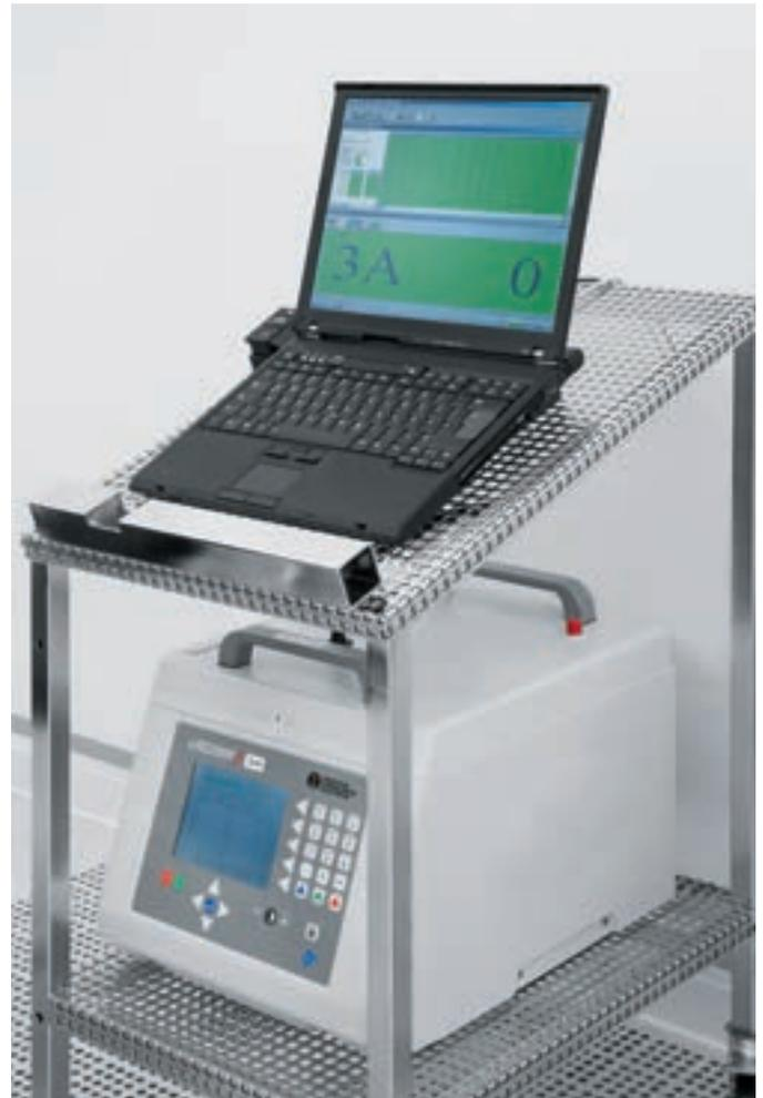
Figure 5: Optical particle counter
