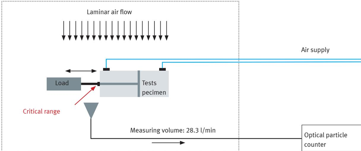
Figure 2: The direct measuring procedure in accordance with VDI 2083-9.1
