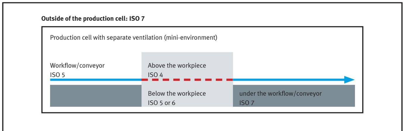
Figure 6: Where a piece of equipment is used is decisive for the required cleanroom class
