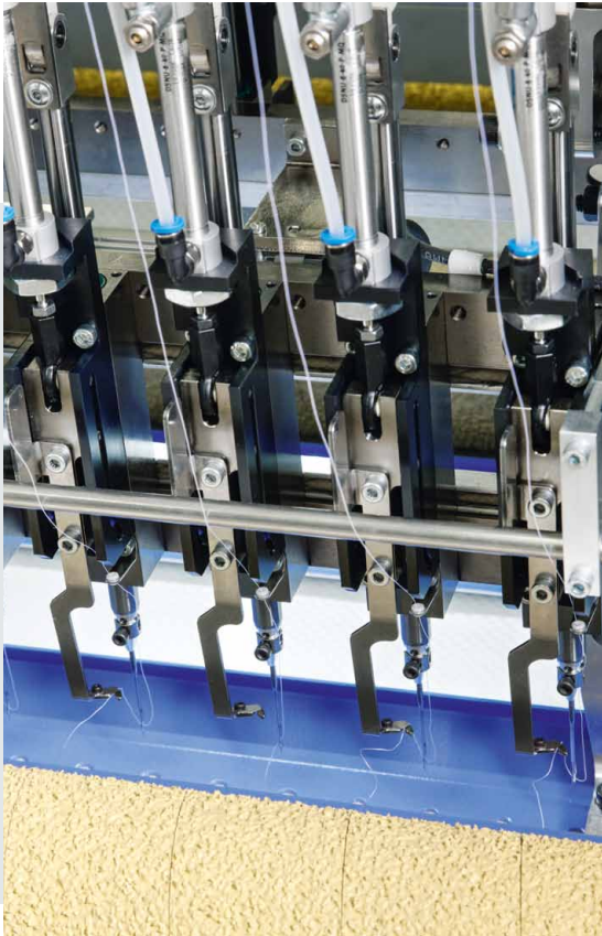
The VMK Select multi-needle quilter uses two rows with up to 96 needles each, each needle capable of 1,600 strokes of minute.
