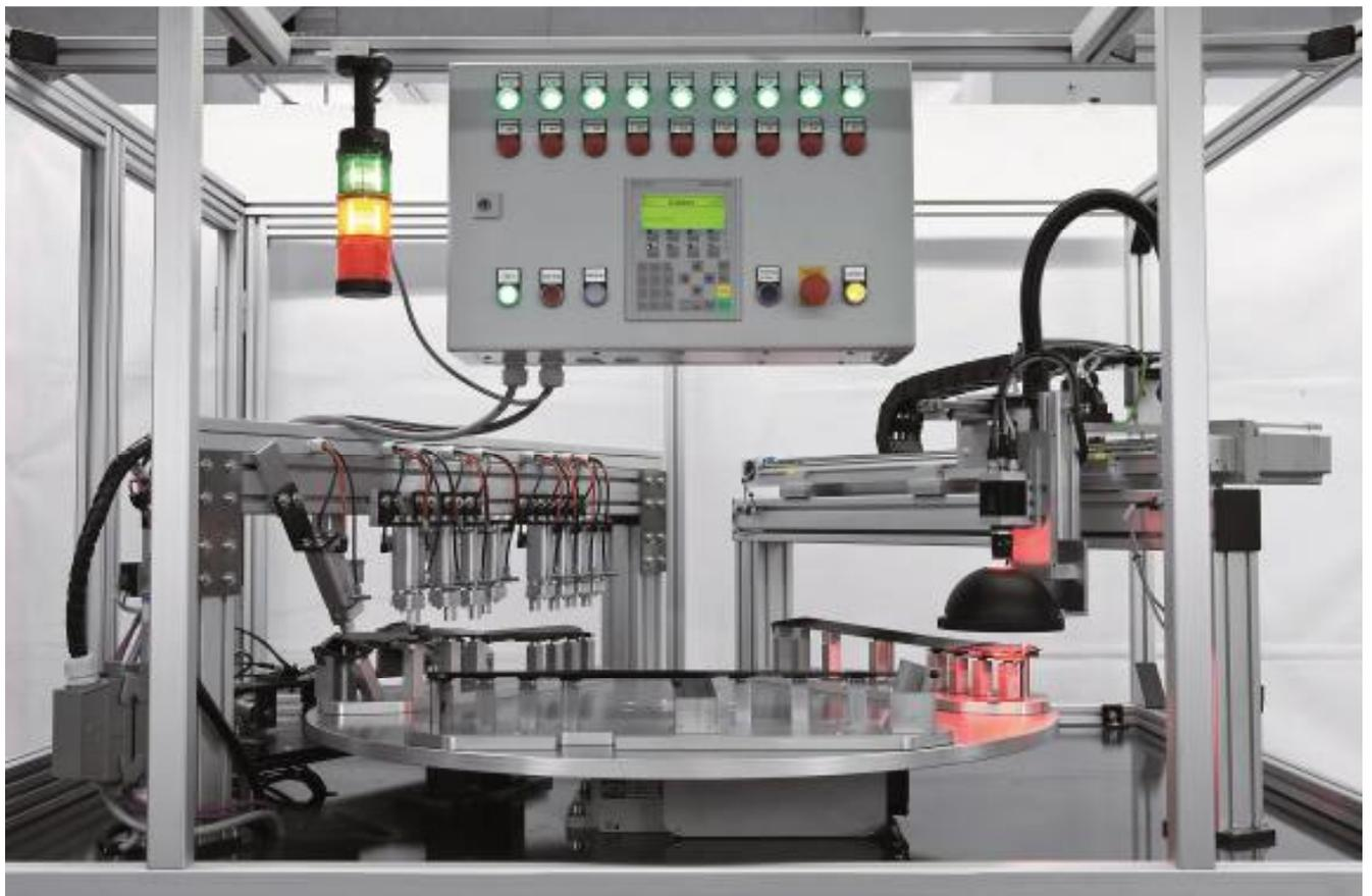
*Getting the green light: 100% inspection of press-fitted plastic sockets in an assembly and inspection cell for an automotive supplier. The vision system travels automatically to each individual position of the sockets. (Photo: Festo)*
