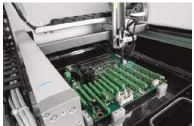
Compact and precise: the compact mini H-gantry EXCM accurately guides the test needle to the test points on the electronic modules.
